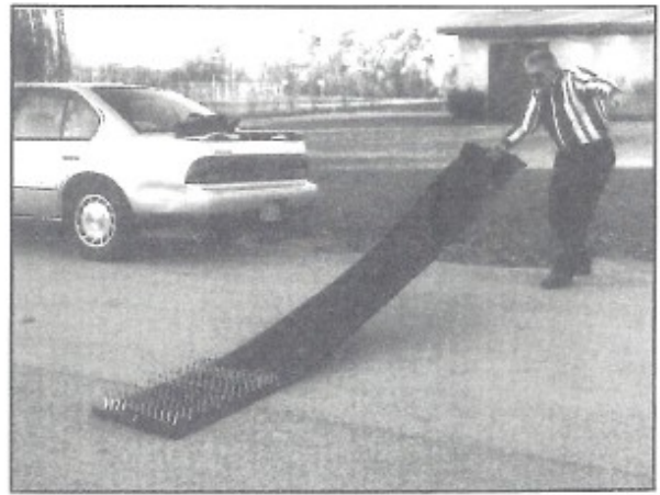
9. The instant the spike assembly hits the ground, take one quick step backwards and...
