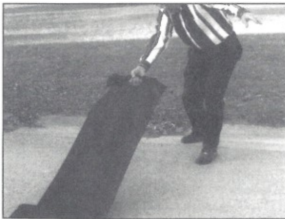
8. Unit will roll forward and hit the ground, unravelling the 12-foot runner wrap.
