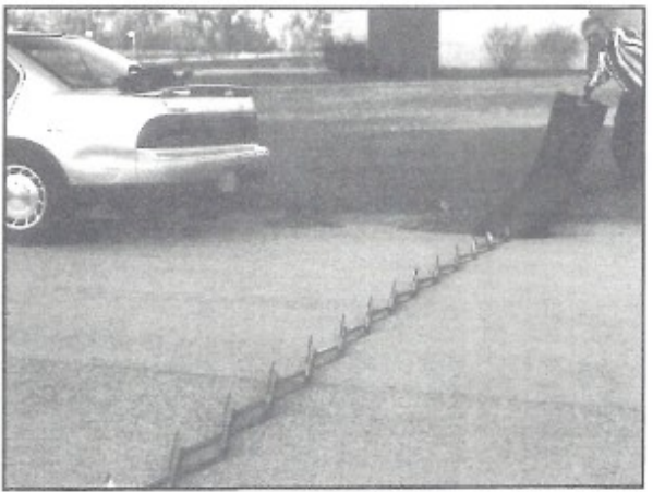
11. This maneuver will shoot the spike assembly to its full 16-foot length.
